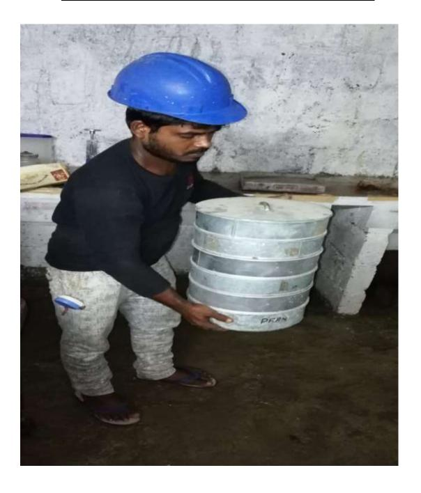
**Fine Aggregate Sieve Analysis Testing**
